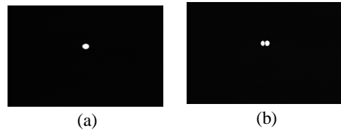
Fig. 2. (a) Only 0 th mode lasing. (b) Only 1 st mode lasing.
